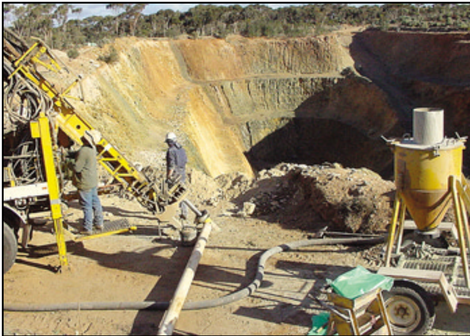
▲ RC drilling at the 5A pit.
