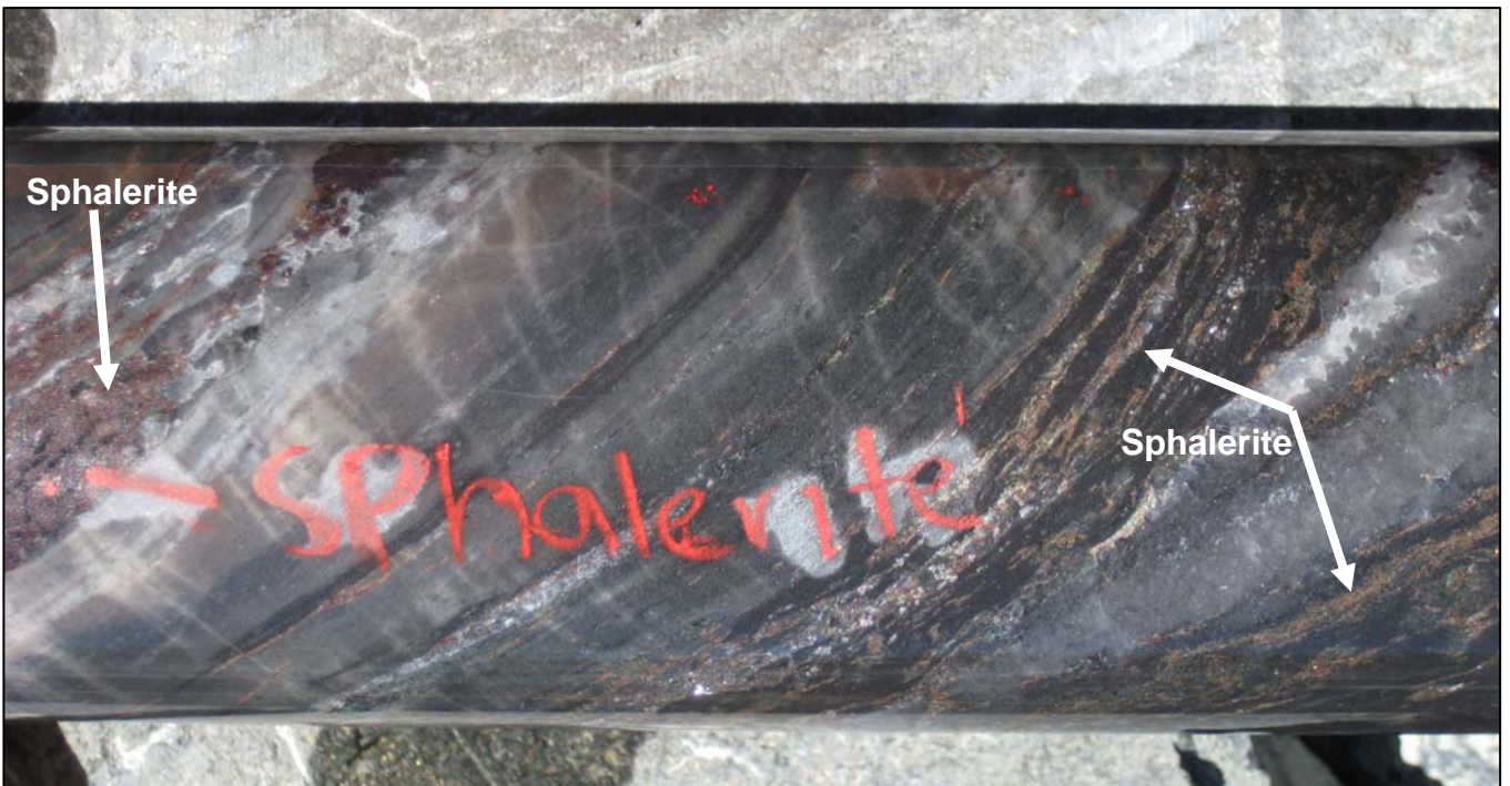
Figure 4: Core Photograph of Representative Zinc Mineralisation in ADD10-06 (length of core sample = 12cms)
